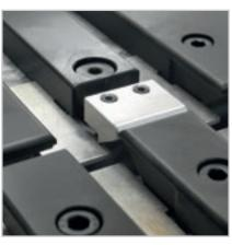
Cutting line closure system, to prevent longitudinal trim cuts from falling into the machine and fouling the blade path.
