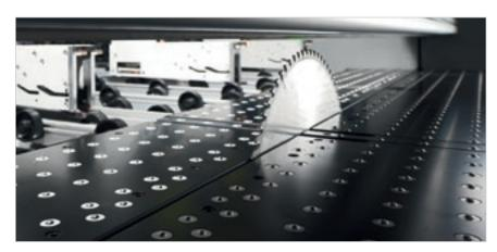
Air-cushioned working surface to handle delicate materials. In addition, this characteristic ensures the surface next to the blade is kept constantly clean.
