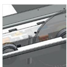
The anti-slide device controls the position and the number of revolutions of the blade, intervening to adjust the advance speed. Maximum cutting quality, a longer blade lifespan, and reduced maintenance costs.
