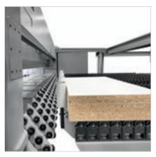
Longitudinal double-edge trims are disposed of by means of a dedicated and fully automated trapdoor with independent rollers.
