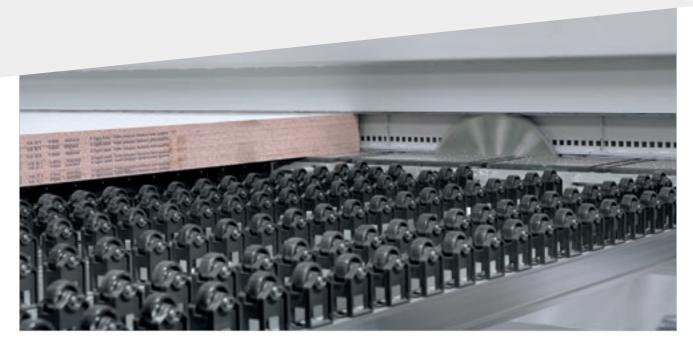
The double presser, with a double, independent structure, enables the application of consistent, controlled pressure to the stack of panels to be cut, thanks to the continuous gripper action, which also creates an actual sealed chamber for trim cuts and an efficient vacuum for the removal of dust.
