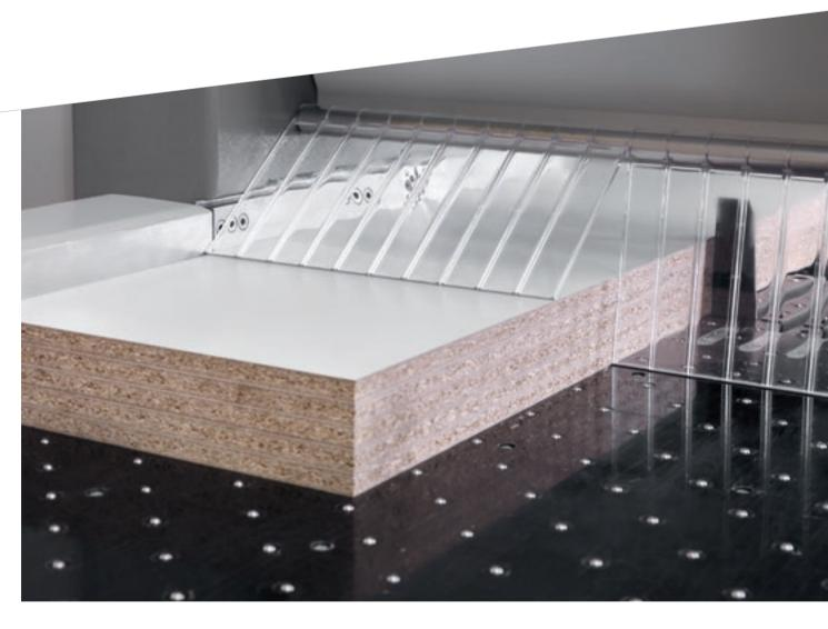
Side alignment stop integrated in the transversal blade carriage. Its features enable the perfect alignment of even the thinnest and/or most flexible panels, reducing cycle time to a minimum
