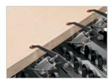
Panel clamping devices avoid the misalignment of the stack during the rotation phase
